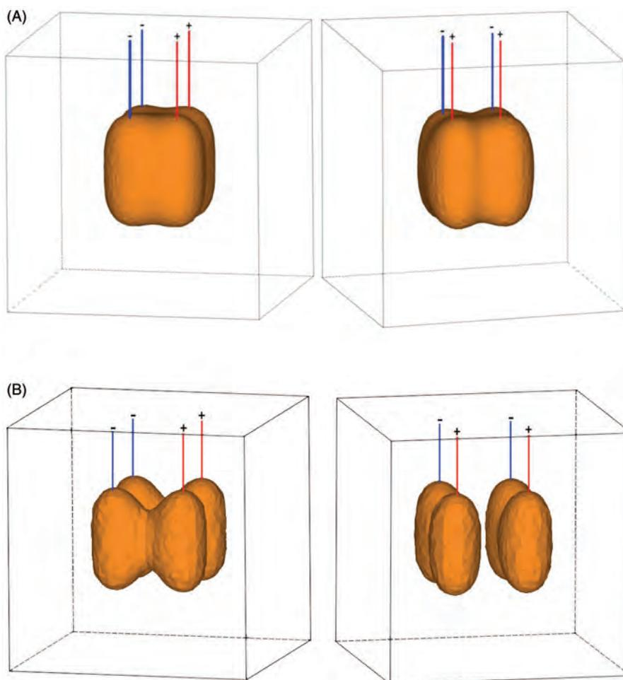
Figure 8. (A) 3D representation of  $50^{\circ}\text{C}$  isotherm after 7 min of RFA applying 50 W with an inter-electrode distance of 2 cm (left: front view; right: side view). (B) 3D representation of  $50^{\circ}\text{C}$  isotherm after 7 min of RFA applying 50 W with an inter-electrode distance of 3 cm (left: front view; right: side view).
