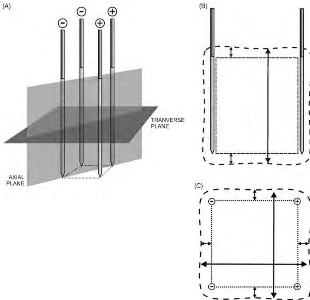
Figure 2. (A) Measurement of the ablation zone size, definition of planes. (B) Measurements in the axial plane: ---- rectangle defined by the active parts of the electrodes; - - - - coagulation zone; small arrows, axial margins outside this rectangle; large arrow, axial diameter. (C) Measurements in the transverse plane: .... square defined by the active parts of the electrodes; - - - coagulation zone; small arrows, lateral margins outside this square; large arrows, transverse diameters.
