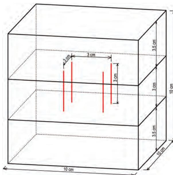
Figure 3. Geometrical model for FEM analysis.
