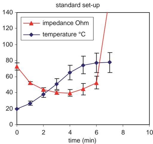
Figure 6. Evolution of impedance and temperature with the standard set-up: 50 W power, 2 cm inter-electrode distance, 1.8 mm diameter electrodes (mean  $\pm$  SD).
