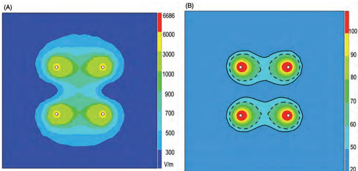
Figure 7. (A) Electric field in the transverse plane at the mid height of the electrodes applying 50 W with an inter-electrode distance of 3 cm. (B) Temperature ( $^{\circ}\text{C}$ ) after 7 min of RFA in the transverse plane applying 50 W with an inter-electrode distance of 3 cm. —  $50^{\circ}$  isotherm; ----  $60^{\circ}$  isotherm.
