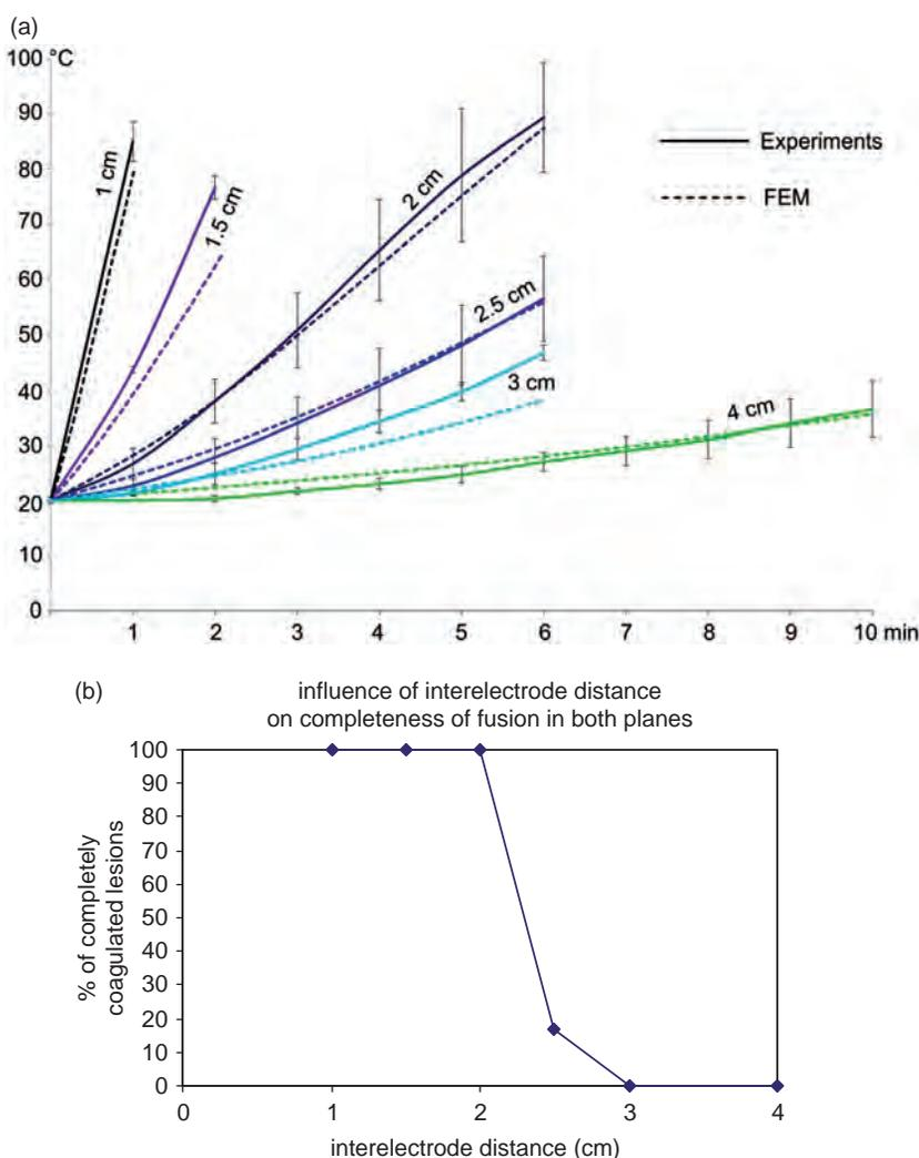
Figure 4. (A) Influence of the inter-electrode distance on temperature as measured during experiments or predicted by FEM. (B) Influence of the inter-electrode distance on completeness of ablation in both planes.
