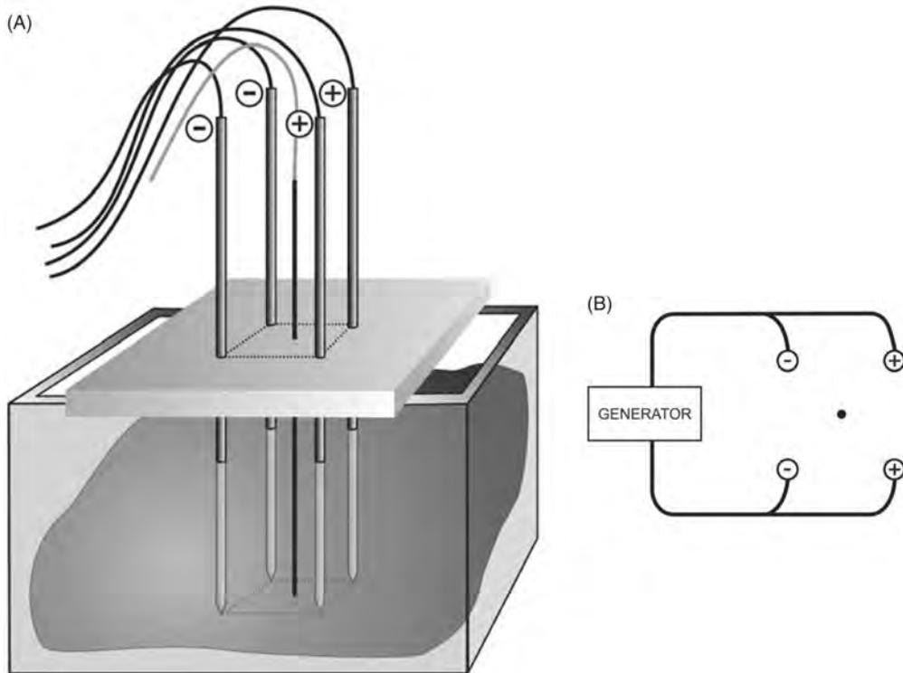
Figure 1. (A) Experimental set-up; (B) Experimental set-up, electric wiring scheme: ○ electrode; ● thermocouple.
